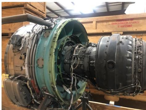
The General Electric CF34 is a turbofan jet engine used on a number of business and regional jets, including the Bombardier Challenger and CRJ series, the Embraer E-Jets, and the Comac ARJ21. First manufactured in 1982, the engine family is in greater demand today than ever before. The engines are currently used around the globe on both military and civilian aircraft operated by SkyWest Airlines, United Airlines, Republic Airlines, Uganda National Airlines Company and more.
