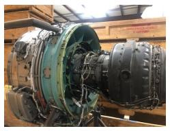
The General Electric CF34 is a turbofan jet engine used on a number of business and regional jets, including the Bombardier Challenger and CRJ series, the Embraer E-Jets, and the Comac ARJ21. First manufactured in 1982, the engine family is in greater demand today than ever before. The engines are currently used around the globe on both military and civilian aircraft operated by SkyWest Airlines, United Airlines, Republic Airlines, Uganda National Airlines Company and more.
